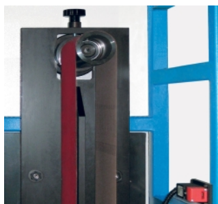
Tensioning of the abrasive belt
